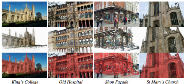
Figure 1: PoseNet: Convolutional neural network monocular camera relocalization. Relocalization results for an input image (top), the predicted camera pose of a visual reconstruction (middle), shown again overlaid in red on the original image (bottom). Our system relocalizes to within approximately 2m and 3° for large outdoor scenes spanning 50,000m 2 . For an online demonstration, please see our project webpage: mi.eng.cam.ac.uk/projects/relocalisation/
