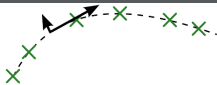
Figure 1: Regularization forces the auto-encoder to become less sensitive to the input, but minimizing reconstruction error forces it to remain sensitive to variations along the manifold of high density. Hence the representation and reconstruction end up capturing well variations on the manifold while mostly ignoring variations orthogonal to it.
